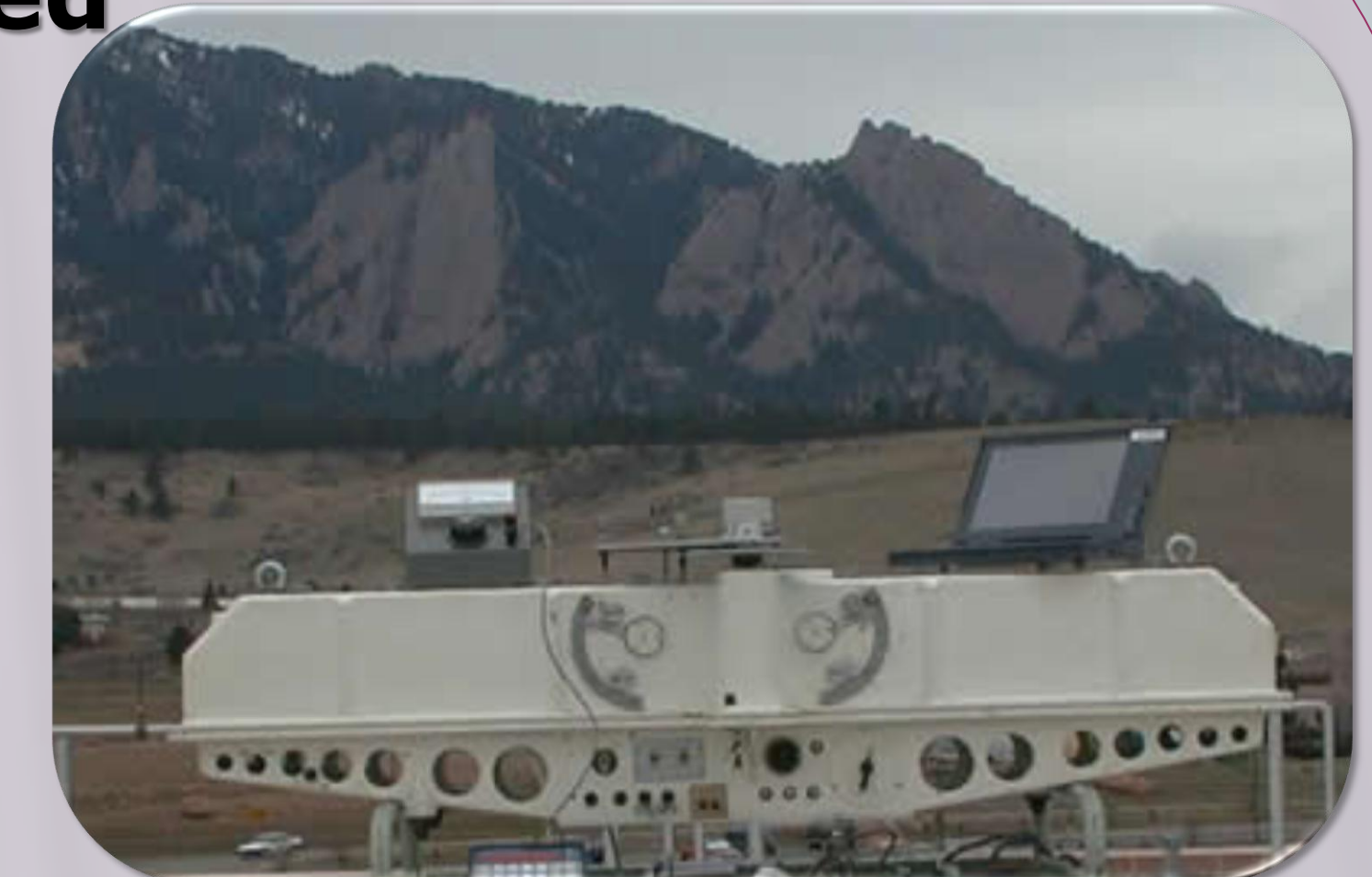
Dobson Spectrophotometer http://ozone.gi.alaska.edu/dobson.htm
